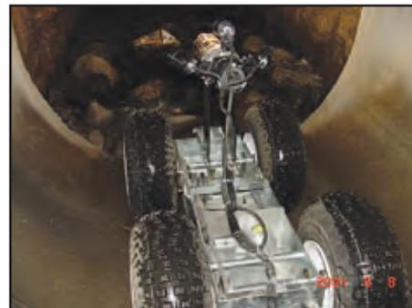
Figure 66: Tractor-mounted camera
