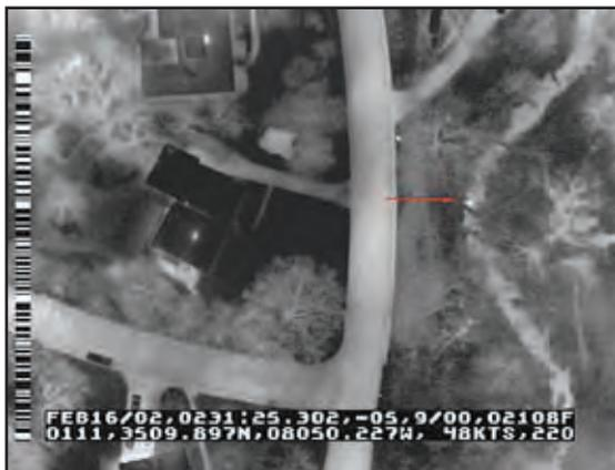
**Figure 72: Aerial thermography showing sewage leak**
