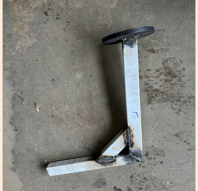
Image 12. Repaired with welding
