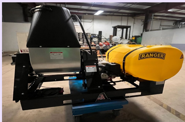
Image 8. Barrier sprayer that will be mounted on the truck
