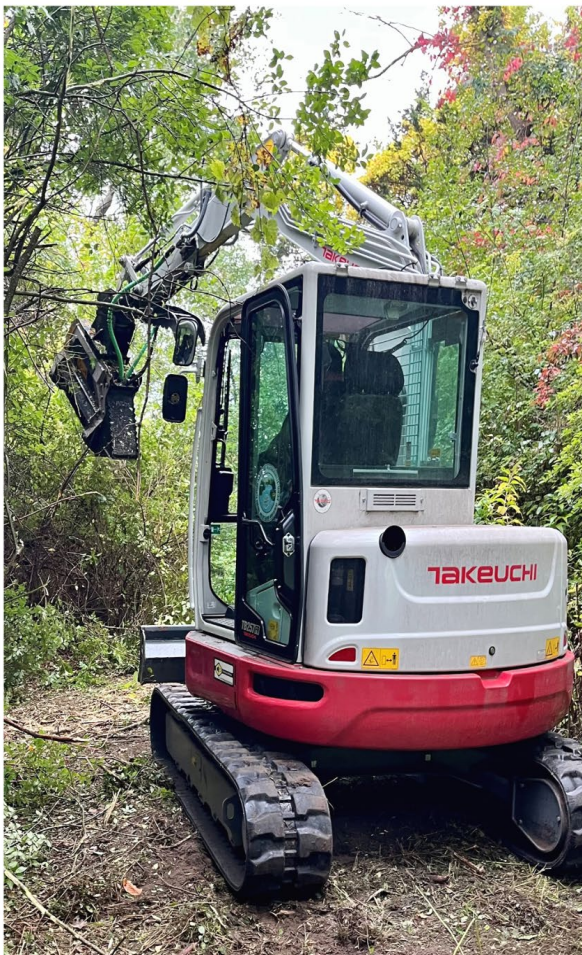
Images 8 and 9. Showcasing how the mulcher can clear through blocked pathways and chew through dead trees.
