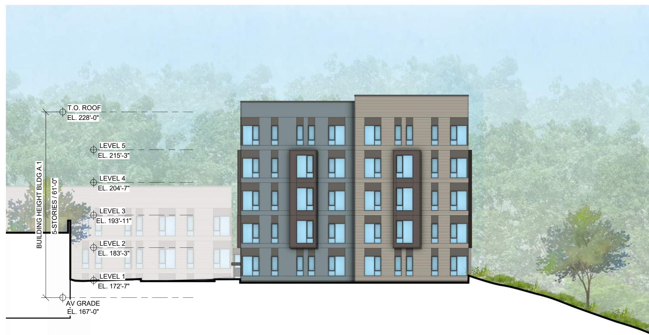
30 EAST ELEVATION - BLDG A Scale: 1/16" = 1'-0"
